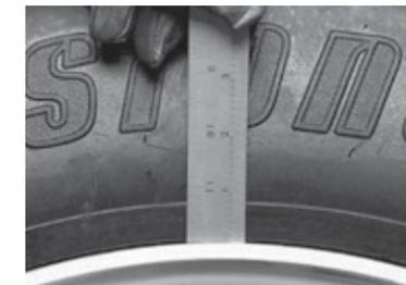
6. Measure distance from molded ring on tire to flange locations, 90 degrees apart.
