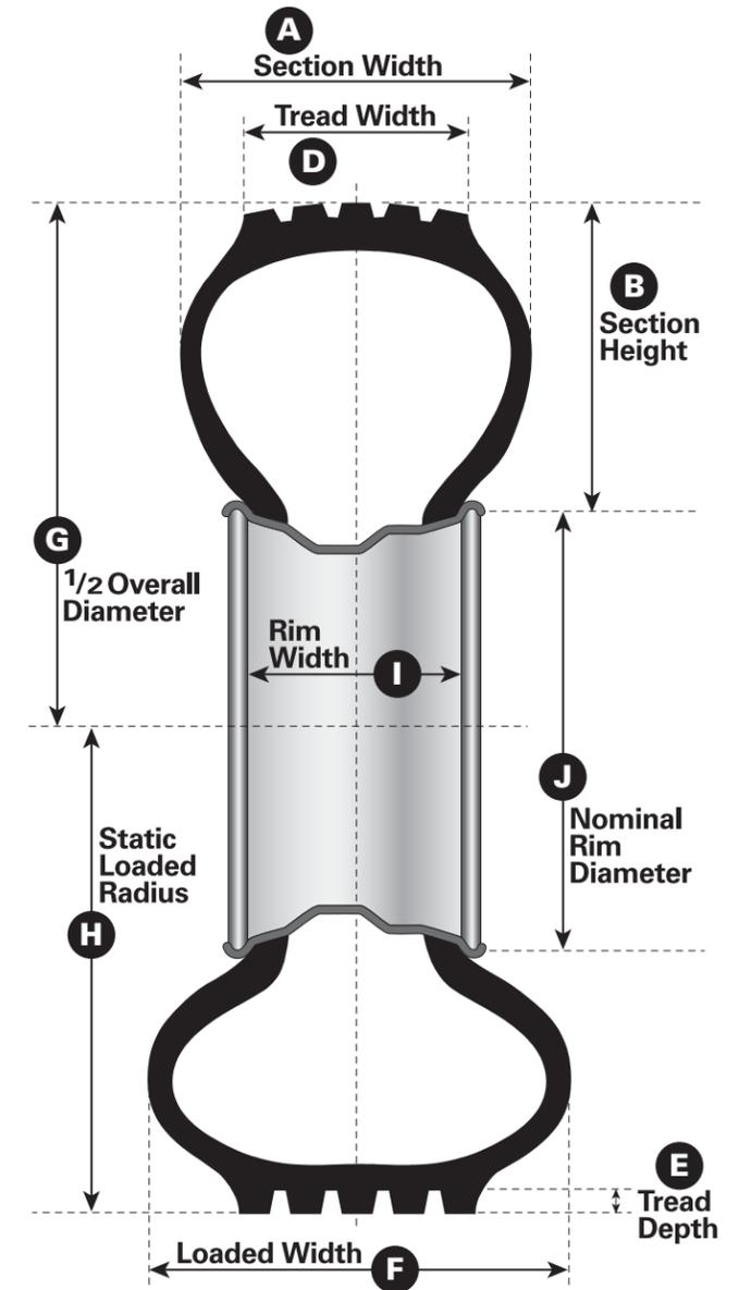
**NOTE: Tires mounted and inflated to recommended pressure. All dimensions measured 24-hours after initial inflation.**
