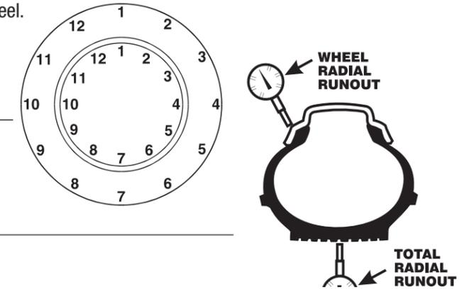
Proper Position for Measuring Runout
