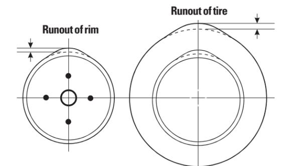
Runout of Tire Due to Runout of Rim
