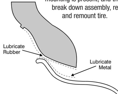
tire sidewall at four locations (90 degrees apart) around the tire-flange circumference. Distances measured should be within a 2/32" (1.5 mm) range for acceptable uniformity. If the ranges in distance within the same side of the tire are greater than this, break down assembly, re-lubricate and remount the tire.
