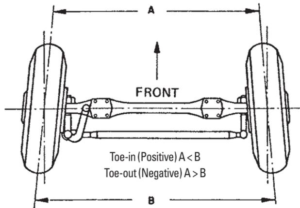
Proper wheel alignment is essential for optimum tire life and vehicle handling characteristics. **Alignment settings should be checked with the truck loaded.** Alignment adjustments can be made on an unloaded truck; however, modifications in the vehicle manufacturer's alignment recommendations may be required for proper "loaded" settings.
