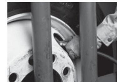
5. Inflate assembly to set bead and check for leaks around the wheel.
