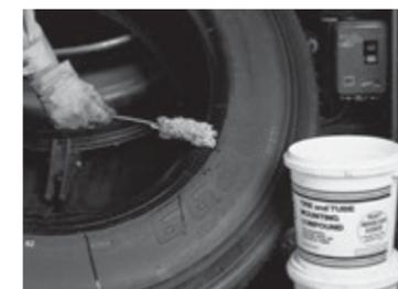
4. Lubricate tire bead. Do not use petroleum or solvent-based products. They cause rubber to deteriorate.
