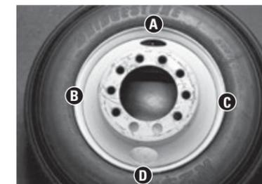
7. Distances A, B, C, and D should be within 2/32". If they are not, break down, re-lubricate and mount again.
