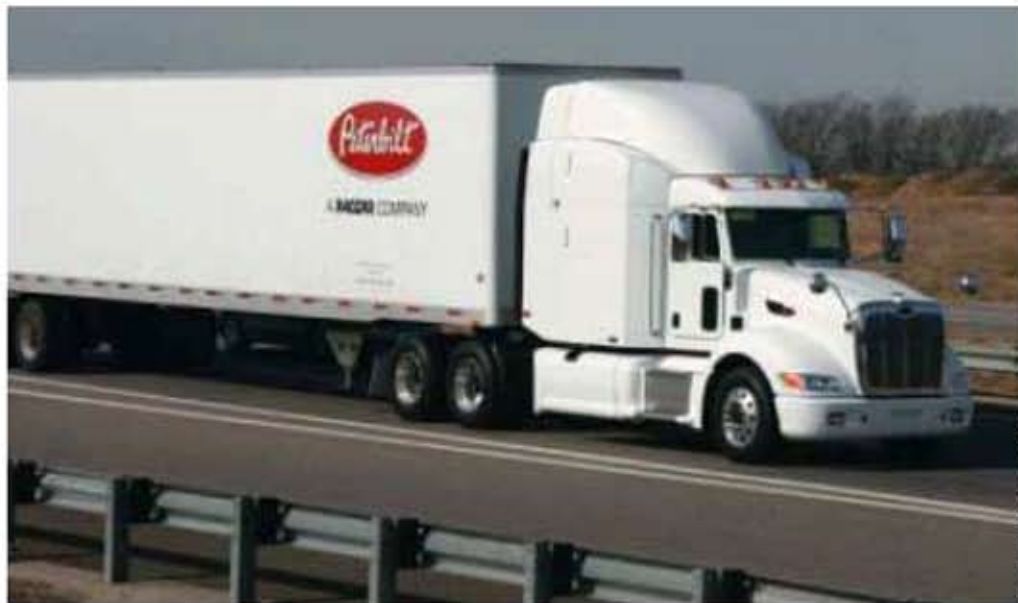
A Model 386 tractor outfitted with the aerodynamic package makes on a test drive at Peterbilt’s technology center in Denton, Texas.
